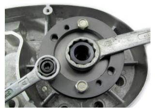
The tool grips the rotor with 2 screws acting as dowels and is held in Position by a SW17 spanner (preferably ring key).
